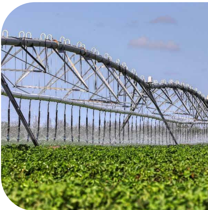
Figure 19: Water Efficient Sprinkler Irrigation System, Medina County, Texas
